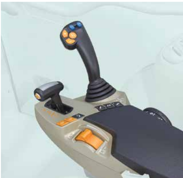
Efficient cab option with electrohydraulic multifunction joystick and armrest
