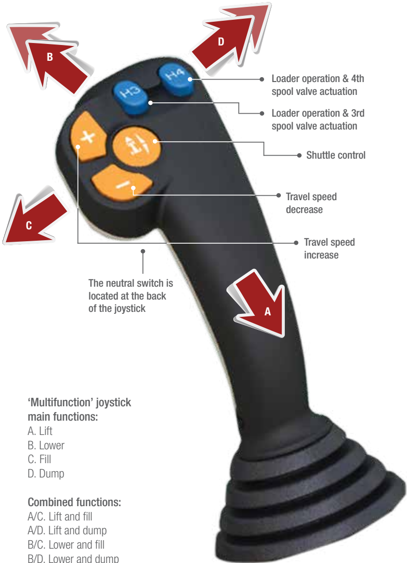
Essential cab option with mechanical multifunction joystick
