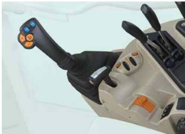
Efficient cab option with electrohydraulic multifunction joystick and armrest
