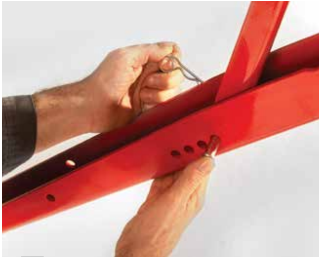
Lower parking stands
