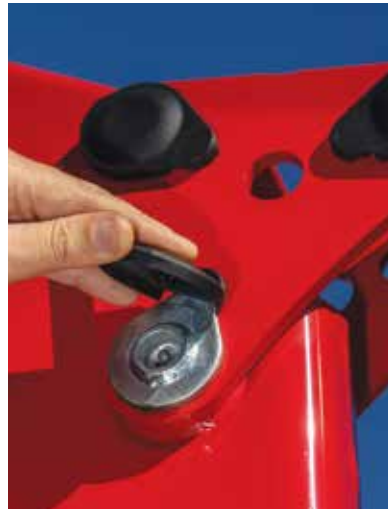
Easy Servicing – outward-facing grease points easily accessible and covered
