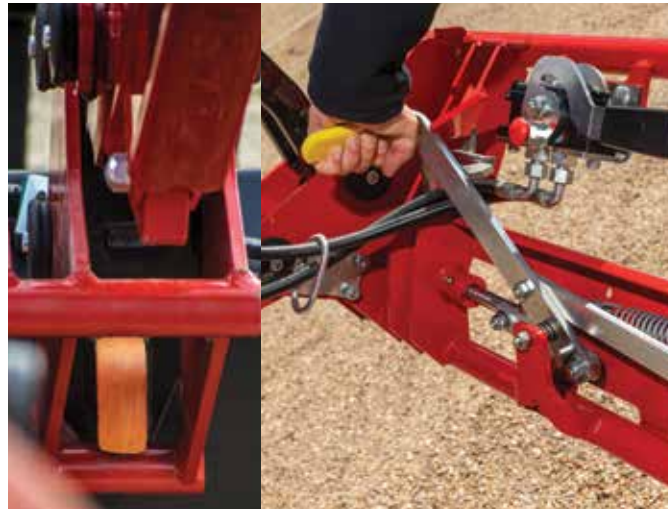
Easy implement changes that increase productivity – In addition to standard Euro tool carrier, a range of optional combi tool carriers are available to allow the use of both Euro implements and a variety of competitive implements.
