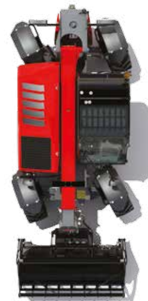
Crab-steer mode - for efficient filling and grading and working alongside walls and in confined spaces.
