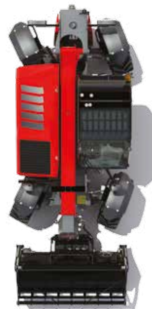
Four-wheel steering mode - for minimum turning circles.
