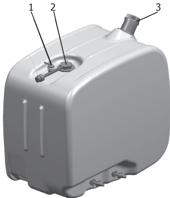
1- breather; 2- combined fluid level and temperature sensor; 3- filling cap cover
