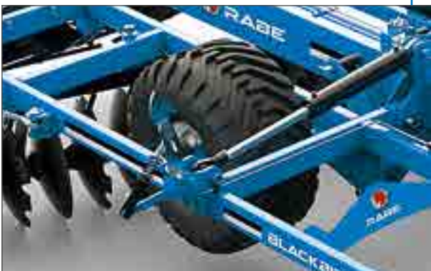
Center axle with hydraulic brakes and depth adjusting.
