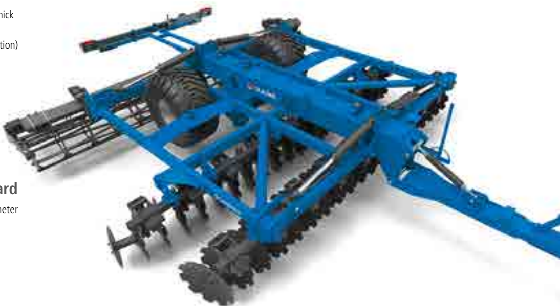
Drawbar low mounted on arms for a better comfort of use.
