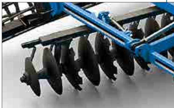
Arrangement of the V-shaped disc trains.
