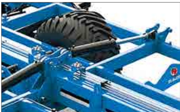
Hydraulic folding for comfortable transport.
