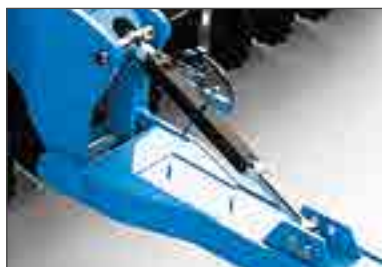
Simple mechanical depth adjustment of the drawbar. Hydraulically as option.
