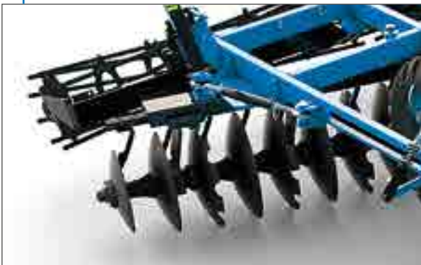
Rear roller for better job finishing and depth adjustment.
