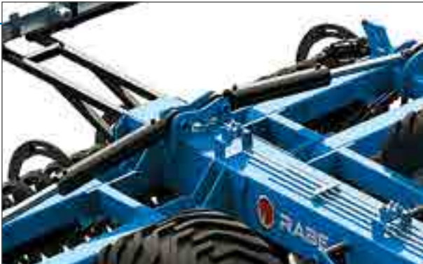
Hydraulic folding for a comfortable transport.
