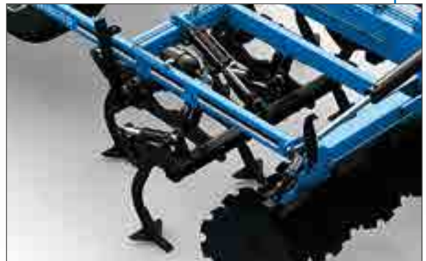
A hydraulic parallelogram adjusts all tines in depth.
