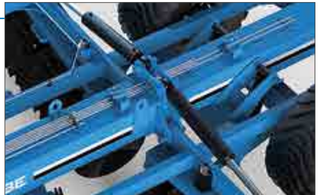
Hydraulic folding for transport.
