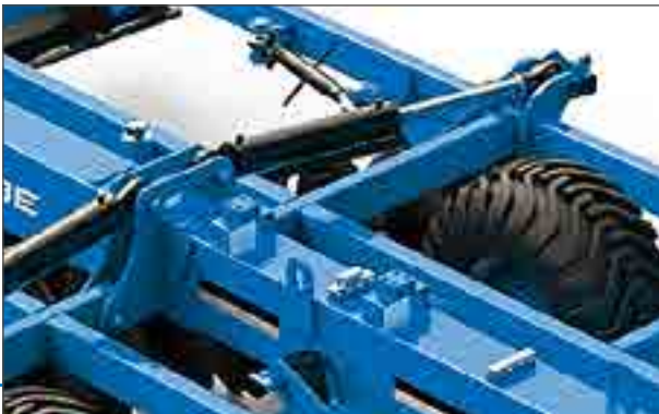
Hydraulic folding for safety and transport comfort.
