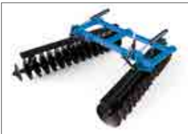
Folding the machines ensures a transport width less than 3.0 m.
