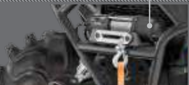
WINCH INSTALLS DIRECTLY TO BUMPER
