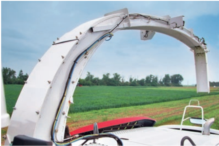
Replaceable silage duct plates reduce time spent on service.
