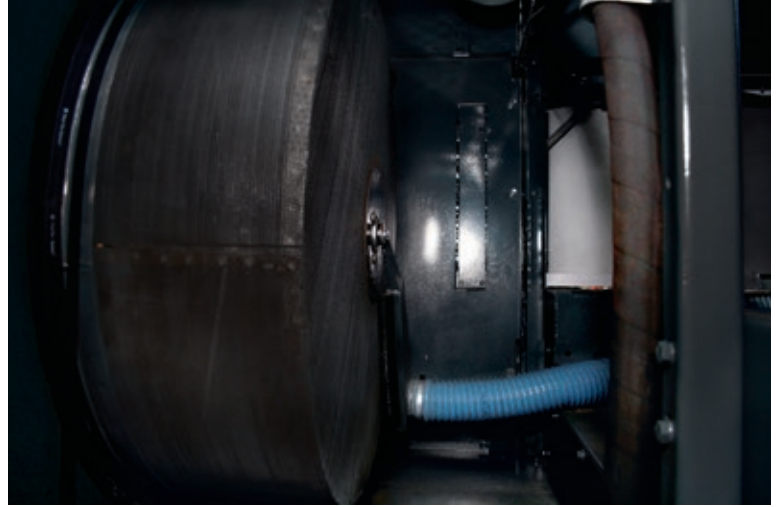
Easy-to-clean radiator screen filter with rotating suction hose.
