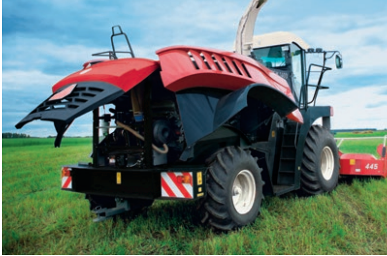
Folding design for convenient maintenance.
